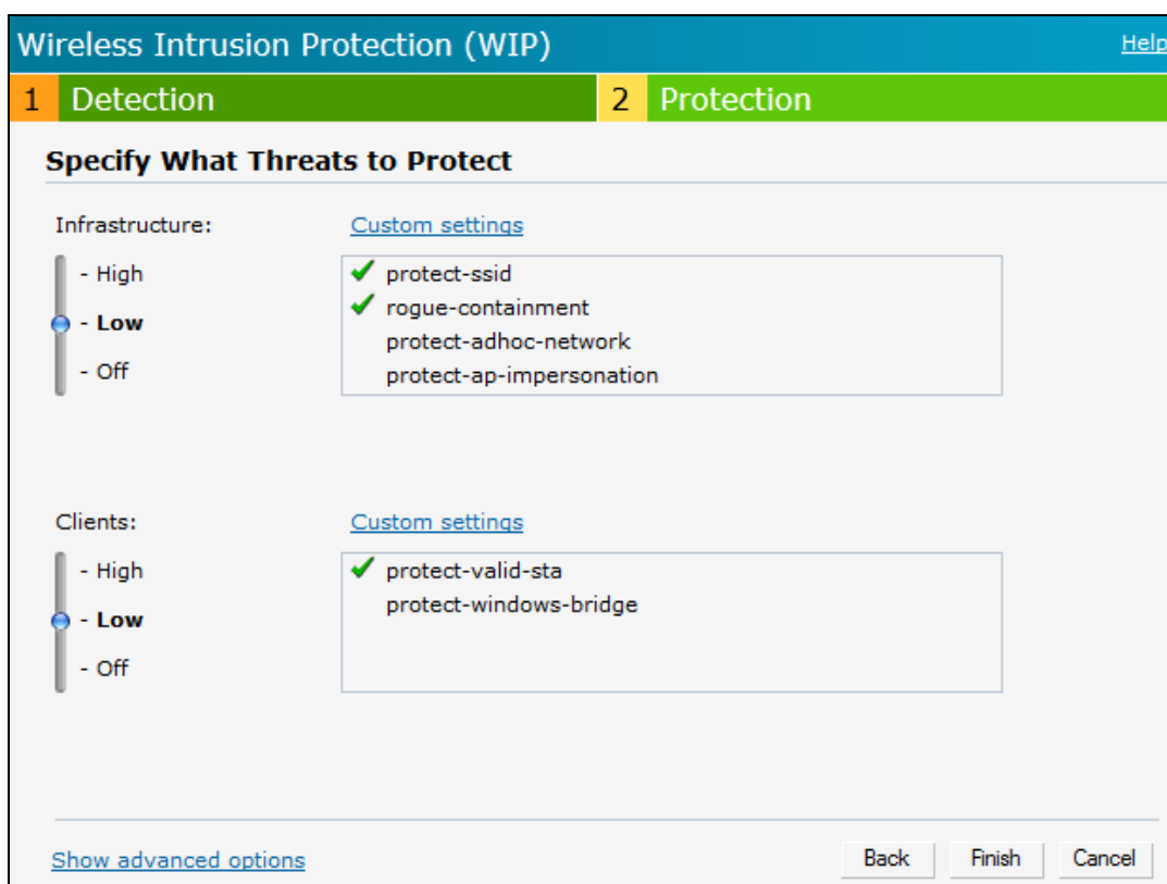
Figure 98 Wireless Intrusion Protection
